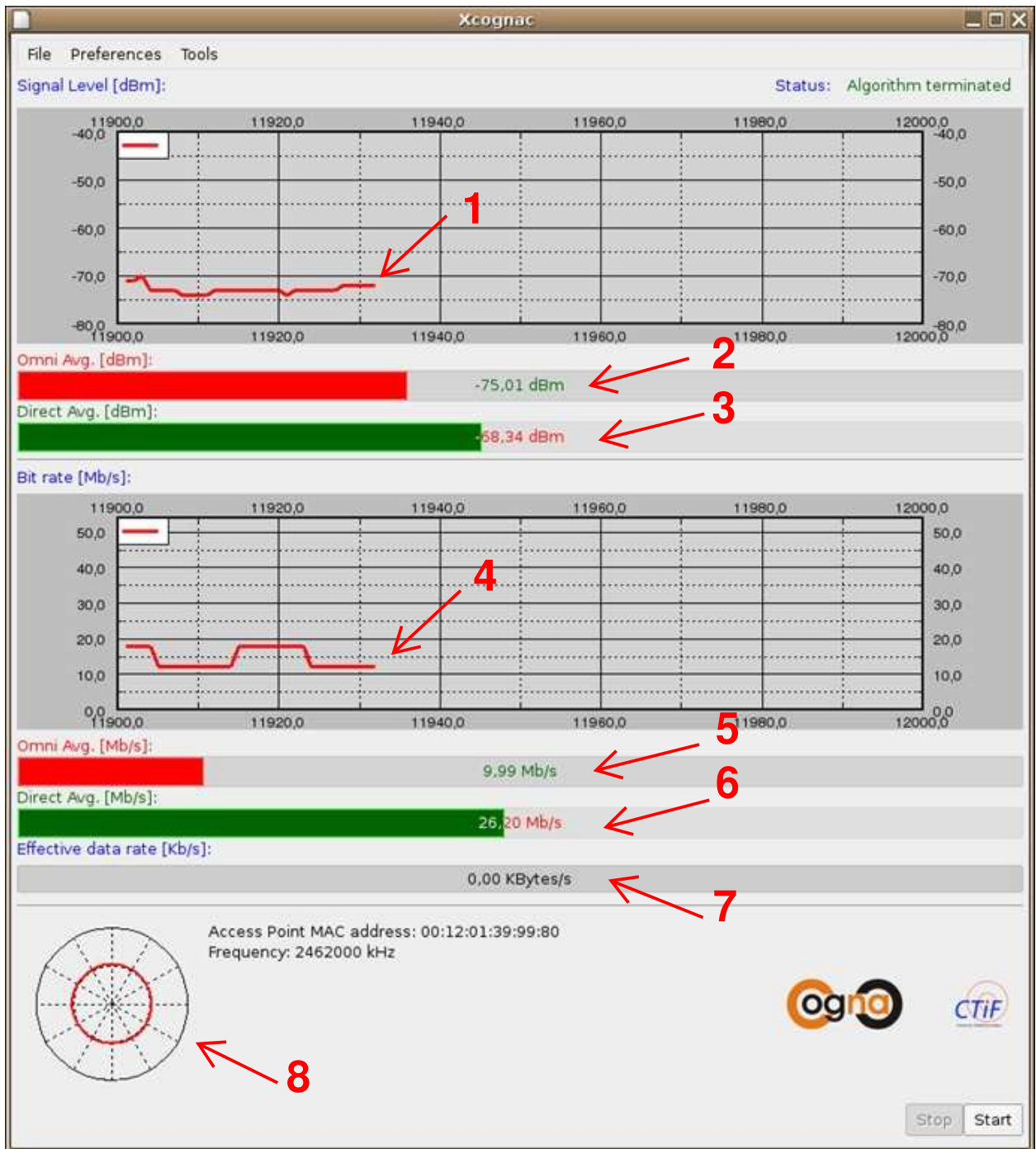
Fig. 5. GUI of the control software showing the monitored information in real time. 1: instantaneous signal strength line, 2: average signal strength bar for the reference case, 3: average signal strength bar for the beamforming case, 4: instantaneous data rate line, 5: average data rate bar for the reference case, 6: average data rate bar for the beamforming case, 7: instantaneous TCP throughput, 8: antenna pattern indicator showing the antenna pattern currently being used.
