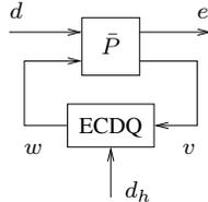
Fig. 6. Entropy coded dithered quantizer inside a feedback loop.
