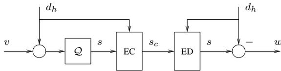
Fig. 5. Entropy coded dithered quantizer.
