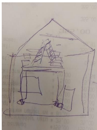
Figure 22: Boris' drawing of self-built scaffolding made of ladder and concrete elements
