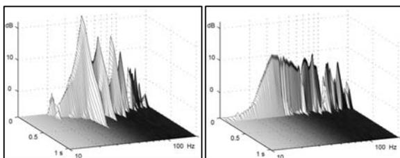
Figure 4. Measured cumulative spectral decay in room A in one point.
