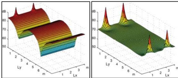
Figure 2. Simulation of 44Hz in room A .
