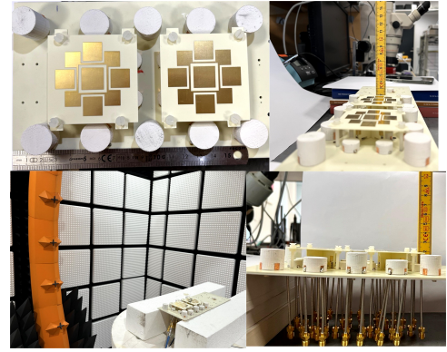
Fig. 18. Prototype of the manufactured subarray
