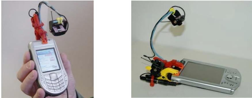
Figure 4. Lightweight camera-clamps attached to mobile devices
