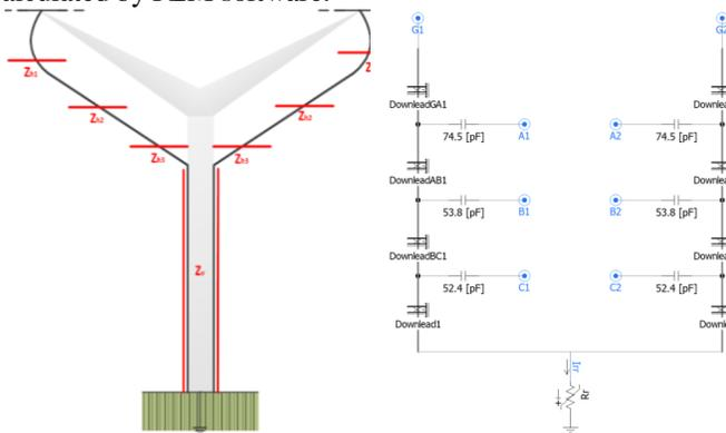
Fig. 3. The demonstration and model of grounding down-leads
