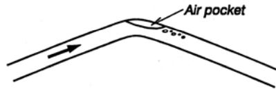
Figure 2.5. Air pocket at a high point.
