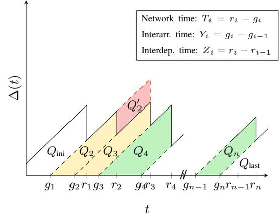
Fig. 4: Evolution of the AoI in a queue network with  $K$  nodes and errors. The network times  $T_i$  are defined as the total time spent in the system, since arrival in node 1 until departure in node  $K$ . The additional area  $Q'_2$ , highlighted in red, shows the increase in the AoI in case a packet is lost.
