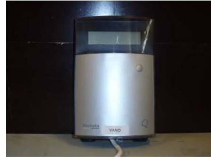
Figure B.0.4: HGQ1 heat consumption measurer.
