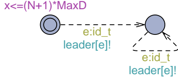
Fig. 9 A property \mathcal{T} stating that a leader is elected within the specified time-bound.
