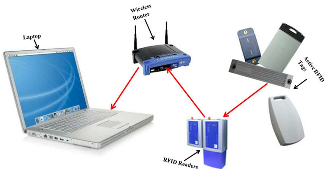
Figure 1: Typical Active RFID Tags and Reader Configuration
