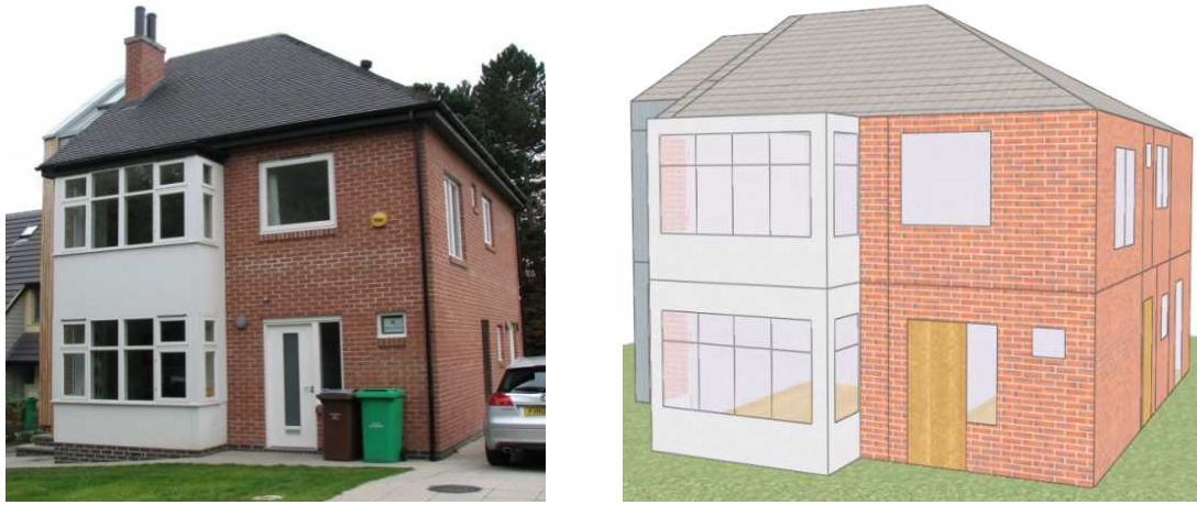
Figure 1 E.ON 2016 house at The University of Nottingham and the IES VE Dynamic Thermal Model
