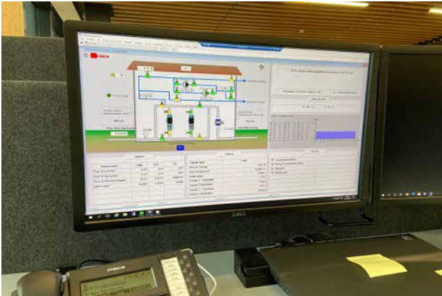
Figure 2. The SCADA system, with a real-time overview over the functioning of a pumping station managed by the water utility of Lemvig (Photo: Jonas Falzarano Jessen)
