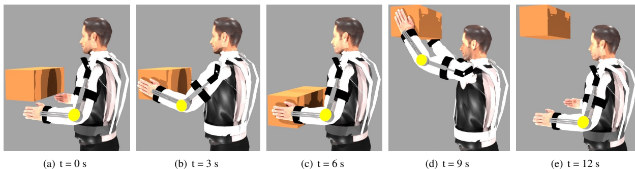
Figure 11. Demonstrations of load lifting task: from time 0 to 3s, the exoskeleton assists the human arm in approaching toward the payload; from 4s to 6s, the human picks the payload and get back to the initial position.; from 7s to 9s, the human arm transfers the payload to a shelf located at a specific height; from 10s to 12s, the human arm gets back to the initial position.
