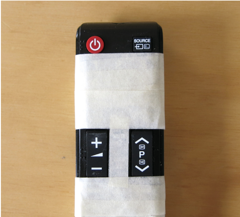
Image 3.1: Remote control with a reduced number of functions
