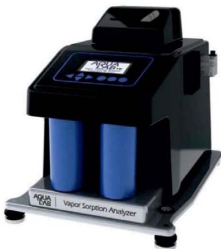
Figure 1. The Vapor Sorption Analyzer (VSA) used to measure water vapor sorption isotherms by the Dynamic Dewpoint Isotherms (DDI) method for the 12 building materials.
