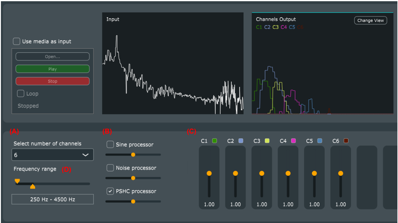
Figure 1. Screenshot of the application in action with a microphone as input source device. The upper section of the layout consists of two displays, visualizing the frequency spectrum of the raw input and processed output; with each channel displayed individually in the output spectrum. The lower section of the layout constitute the user-configurable parameters, and can be modified to adjust the output in real-time. Use (A) to select number of channels, (B) to enable and disable carrier types, and control the gain of each carrier, (C) to control the gain of each individual channel, and (D) to adjust the upper and lower cut-offs of the frequency range in which the band-pass filters will be distributed between.
