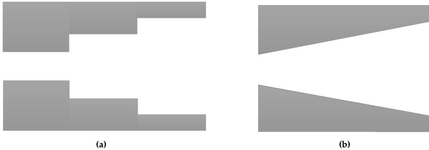
**Fig. 1.7:** Illustration of a microchannel featuring a) Stepped diverging and b) Smooth diverging cross-section. The flow enters from the left and exits on the right in both designs. Adopted from Yahyaee et al. [4] © 2019 IEEE.
