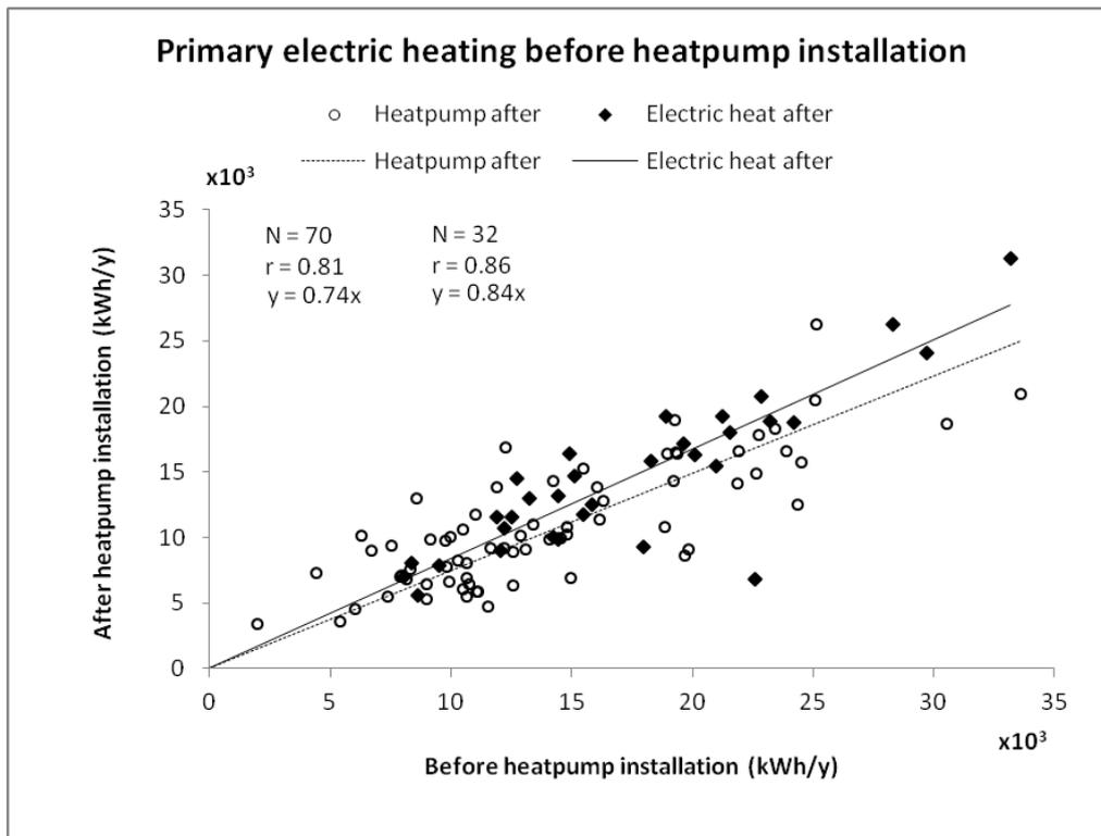
**Figure 3.** Comparing annual household electricity consumption before and after a heat pump was installed for households that used direct electric heating before and distributed on what type of heating they used afterwards. Electricity consumption for heating is corrected for degree days.
