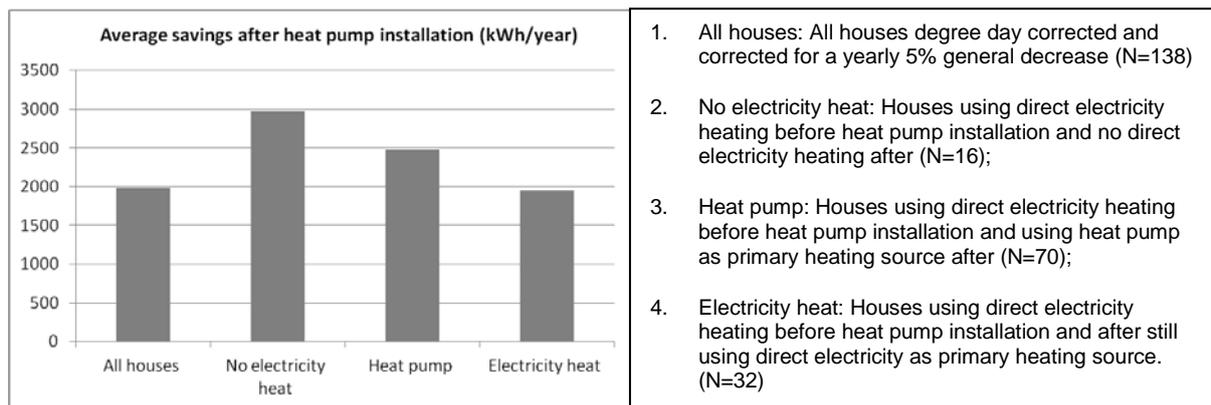
**Figure 2.** Average savings in annual household electricity consumption (kWh) before and after heat a pump was installed, for different combinations of heat supply before and after installation of a heat pump. For all four cases, the savings differ significantly from zero.
