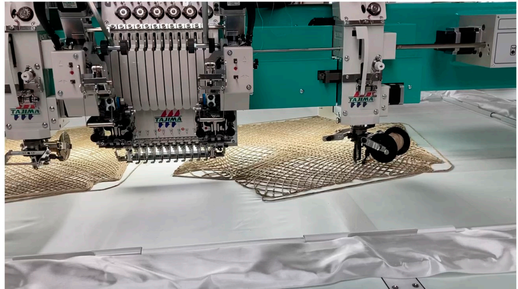
Figure 3. Tailored Fiber Placement (TFP) of flax fibers. ©BioMat.
