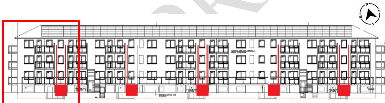
178 Figure 1: The South façade of the case study where the red rectangles are the approximate locations of the GSHP in 179 separate technical rooms.
