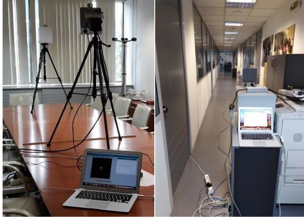
Figure 4-1 Indoor LoS measurements setup: (a) a conference room setup with a distance of 2–6m between Tx and Rx (b) Measurements in the corridor where the distance between Tx and Rx is 20m.
