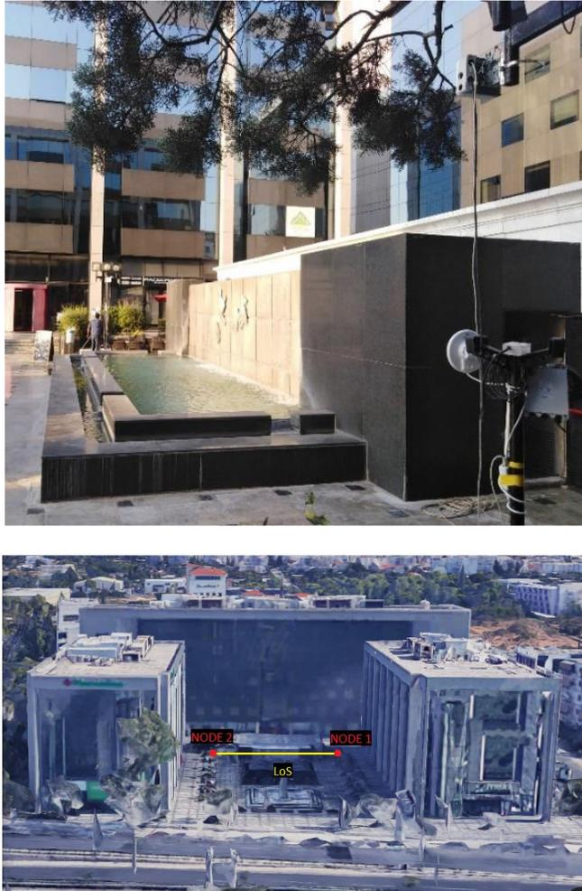
Figure 4-4 Outdoor-outdoor propagation measurements setup for the Facebook sounder nodes in urban environment outside monumental plaza, where both sounder nodes are mounted on lamp posts. The measurements are carried out across a water fountain to see the reflections and the scattering.
