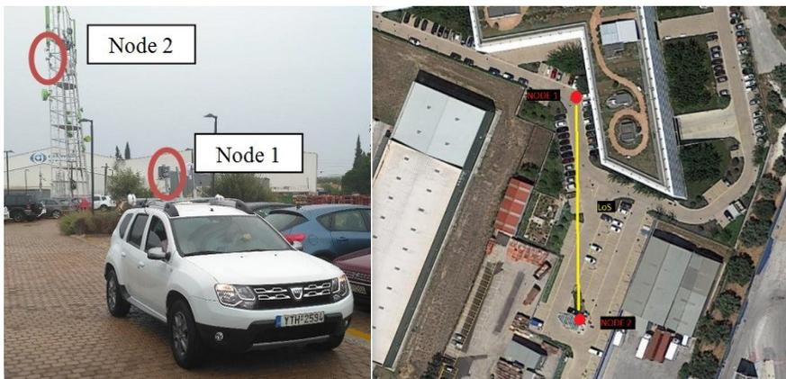
Figure 4-3 Outdoor-outdoor propagation measurements setup for the Facebook sounder nodes in suburban environment, where one sounder is mounted on a commercial telecom provider COSMOTE's tower and the second node is on the roof of a moving SUV.
