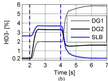
Fig. 8. (a) DGs and SLB voltage unbalance factor, (b) DGs and SLB voltage distortion index for 3<sup>rd</sup> harmonic negative sequence.
