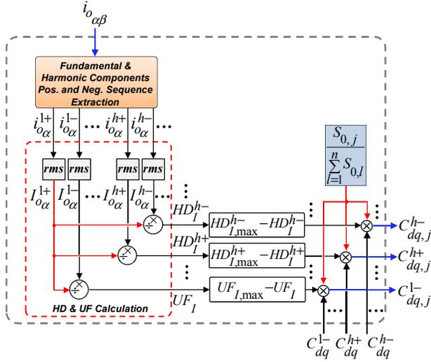
Fig. 6. Block diagram of compensation effort controller of DG<sub>j</sub>.
