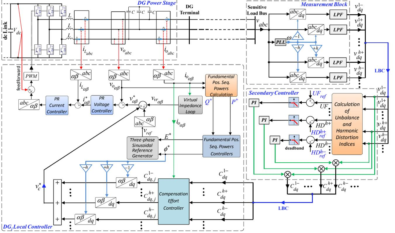
Fig. 2. Detailed block diagram of the control system.
