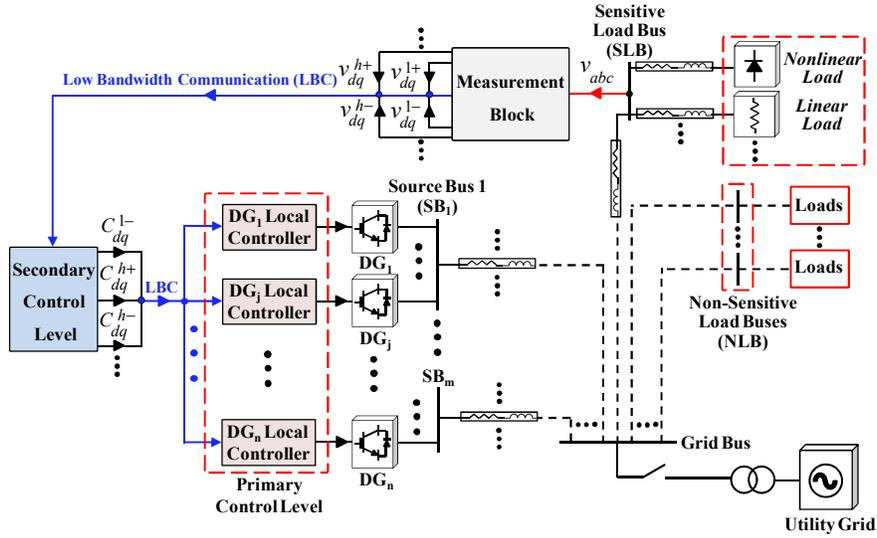
Fig. 1. Hierarchical control scheme for a general microgrid.
