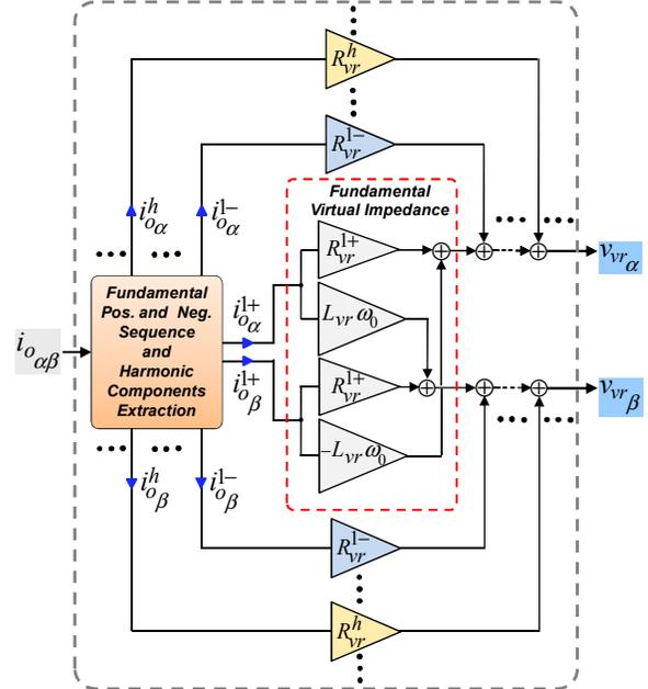
Fig. 5. Block diagram of selective virtual impedance.
