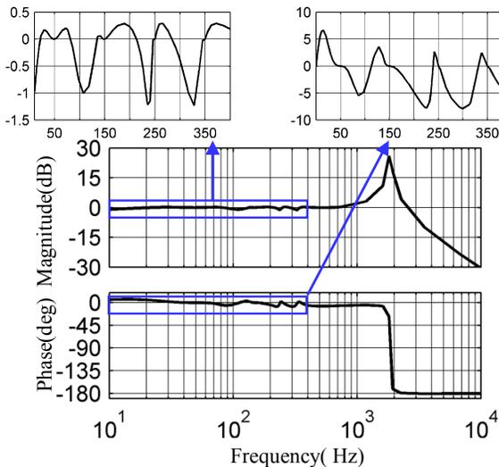
Fig. 3. Bode diagram of closed loop transfer function.
