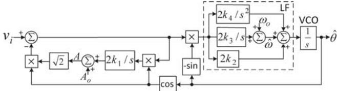
Fig. 4. Basic scheme of the type-3 EPLL.
