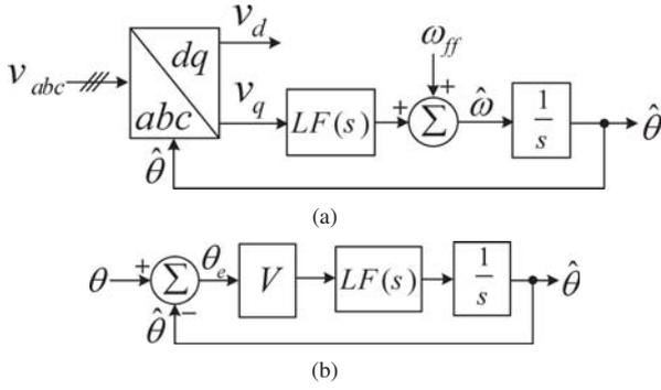
Fig. 2. (a) Basic scheme of a conventional SRF-PLL, and (b) its small-signal model.
