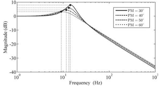
Fig. 12. Closed-loop Bode magnitude plots for different values of PM.
