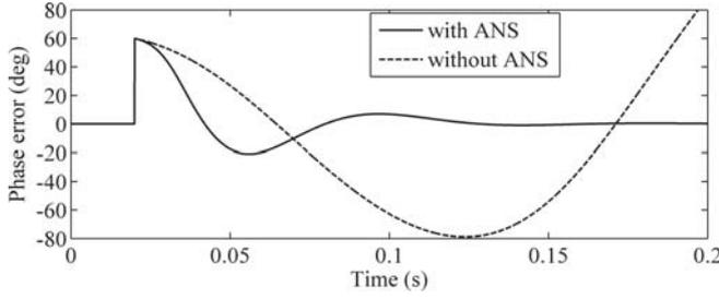
Fig. 17. PLL phase-error response to a voltage sag of 0.9 pu associated with a phase-angle jump of  $60^\circ$ .
