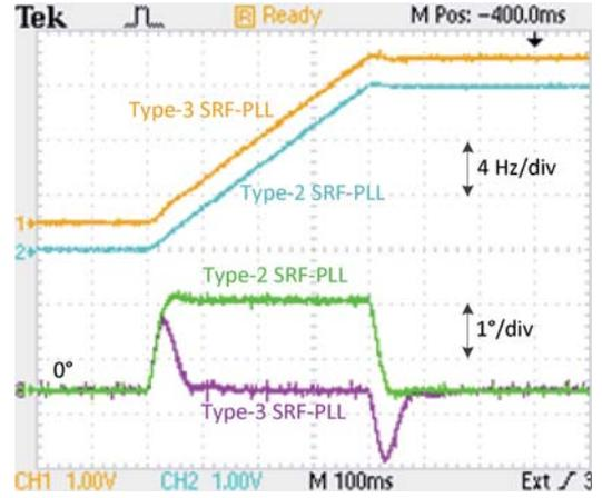
Fig. 24. Experimental results when the grid voltage frequency changes linearly with time at a rate of  $\Delta\omega = 2\pi 30 \text{ rad/s}^2$ : Ch1 and Ch2 denote the estimated frequency (4 Hz/div), and Ch3 and Ch4 denote the phase error (1°/div).
