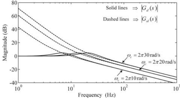
Fig. 13. Bode magnitude plots of  $G_d(s)$  (solid lines) and  $G_{ol}(s)$  (dashed lines) for three different values of  $\omega_c$ .
