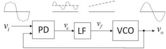
Fig. 1. Basic scheme of a typical PLL.
