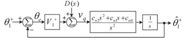
Fig. 9. Small-signal model of the type-3 SRF-PLL.
