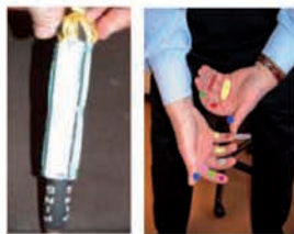
Figure 1: Pressure sensors at the grasp of the golf club (left) Analyzed pressure areas at the left and right hand (right)
