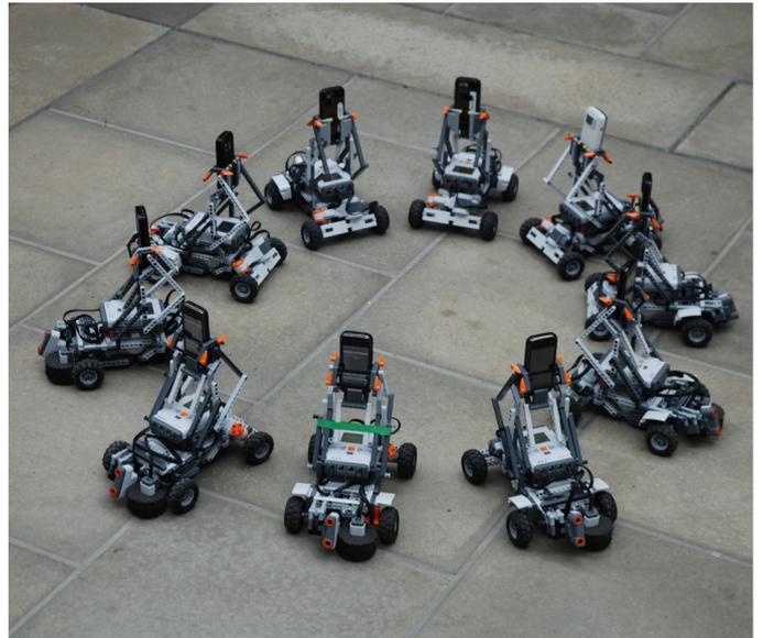
Figure 2. LEGO robots carrying 10 Nokia mobile phones
