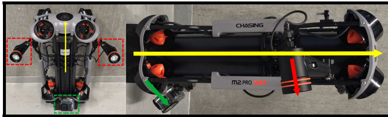
Fig. 10: The underwater ROV captured from two different angles. The position and orientation of the camera and light sources are highlighted by green and red markings, respectively. The yellow arrows indicate the forward orientation of the drone.
