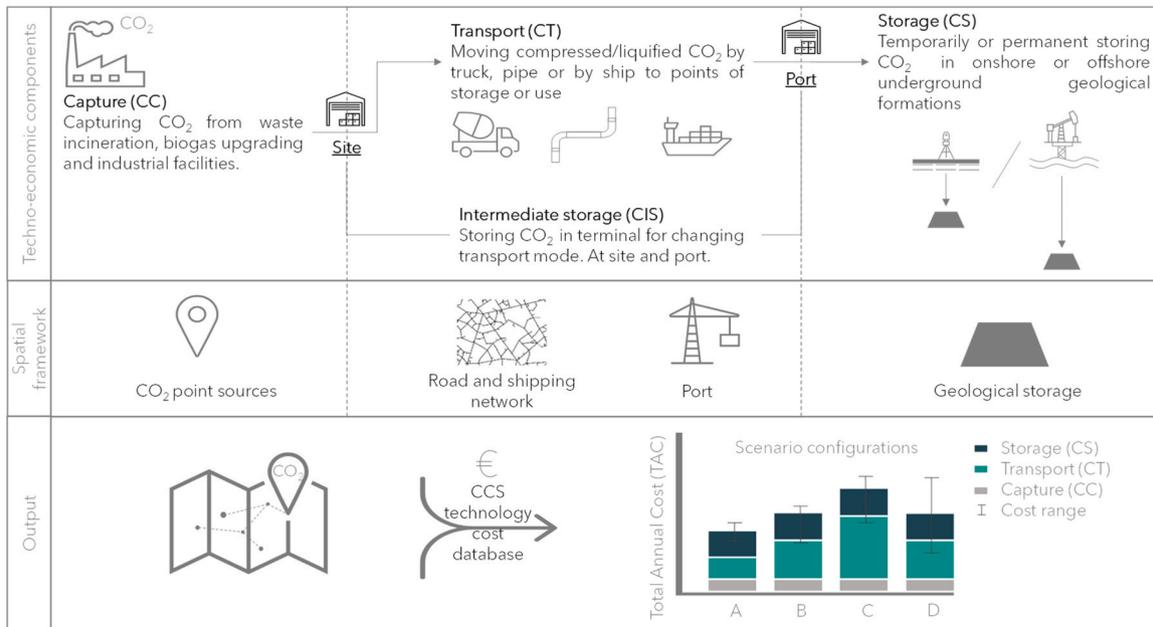
Fig. 1. Geographical CCS cost model: Components and output overview.
