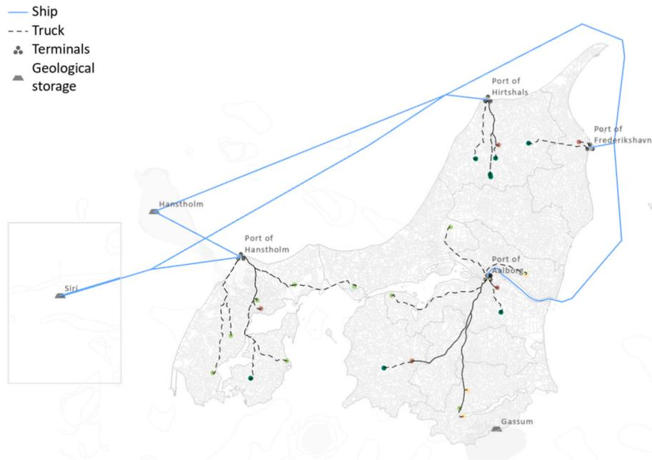
Fig. 7. Scenario A: Offshore storage geographical routing via truck and ship.
