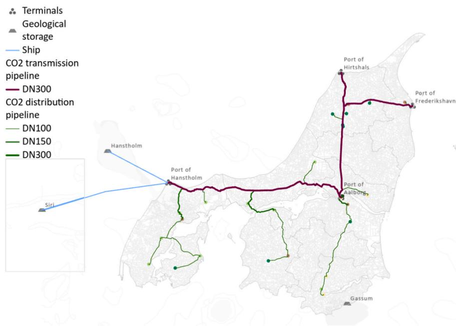
Fig. 8. Scenario B: Offshore storage geographical routing via pipeline and ship.
