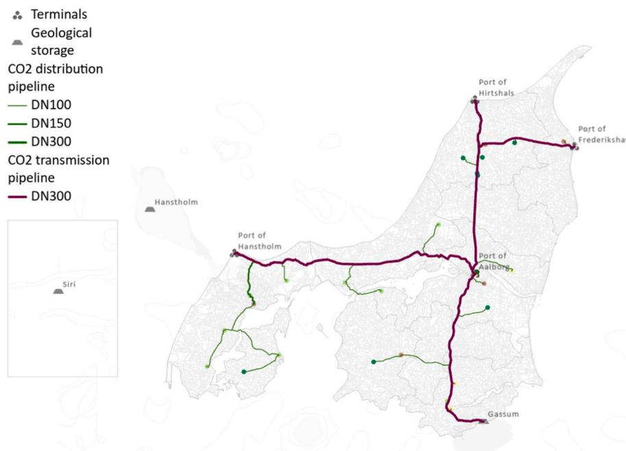
Fig. 10. Scenario C: Onshore storage geographical routing via pipeline.
