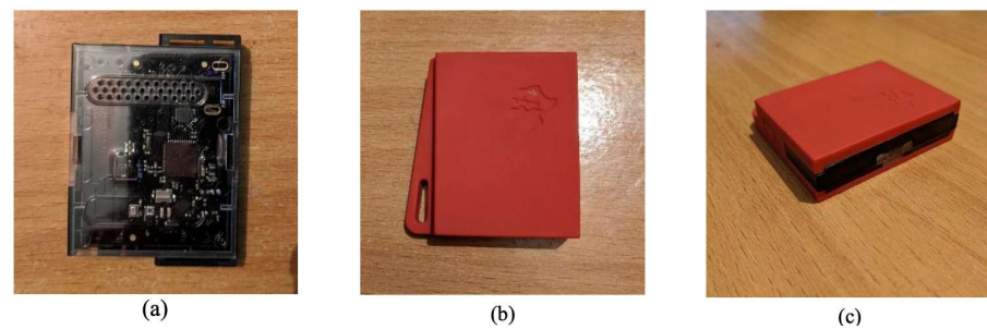
Figure 3. The TI CC2650 Sensor Tag IoT module. (a) Circuit clearly visible with cover removed, (b) view from the top with cover intact, (c) side view with on/off button [44].
