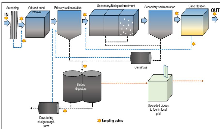
Figure 7: Flow diagram of Käppala WWTP and sampling points.
