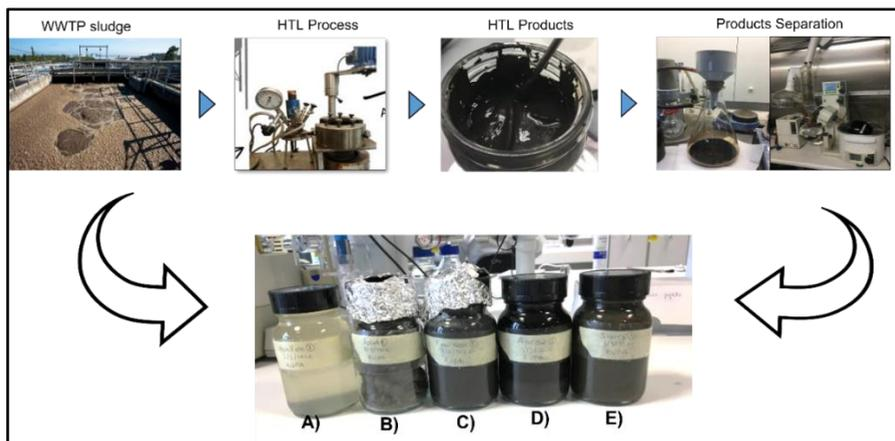
Figure 6: Sewage sludge treated with hydrothermal liquefaction (HTL) process and separation of the received products into different forms: A) Distillate water, B) Solid residue, C) Emulsion, D) As-received product from HTL chamber, and E) Slurry.
