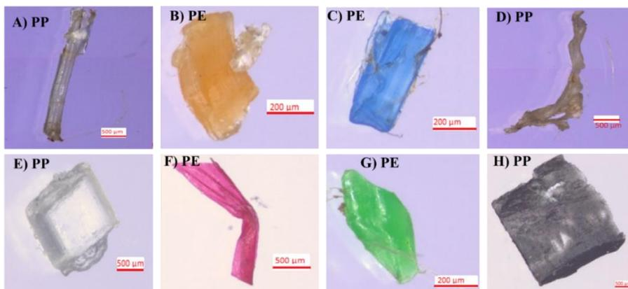
Figure 5: Microplastics (> 500  $\mu\text{m}$ ) analyzed with ATR-FTIR.
