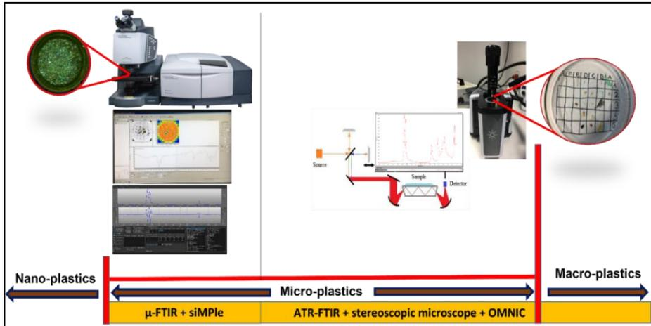
Figure 3: Used analytical techniques (Agilent Technologies) to analyze microplastics (10 – 5000  $\mu\text{m}$ ) in the present study.
