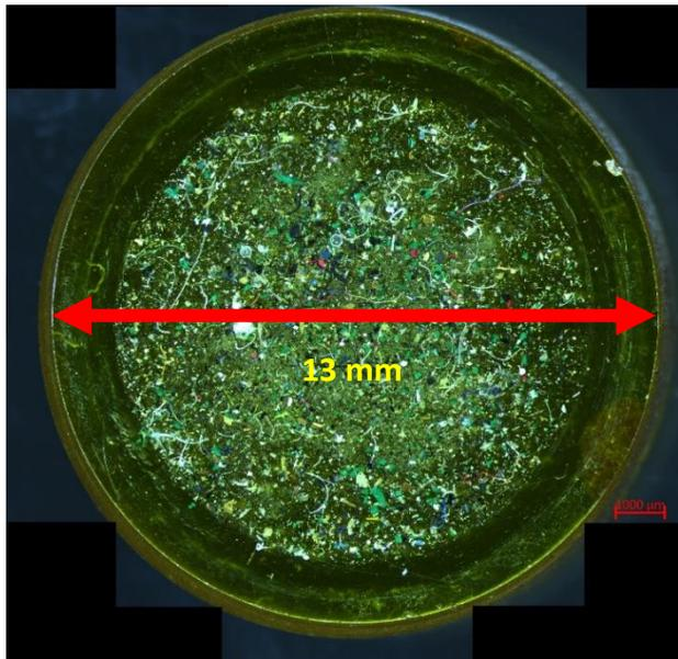
Figure 4: Microplastics (10 - 500  $\mu\text{m}$ ) analyzed with FPA- $\mu$ -FTIR.
