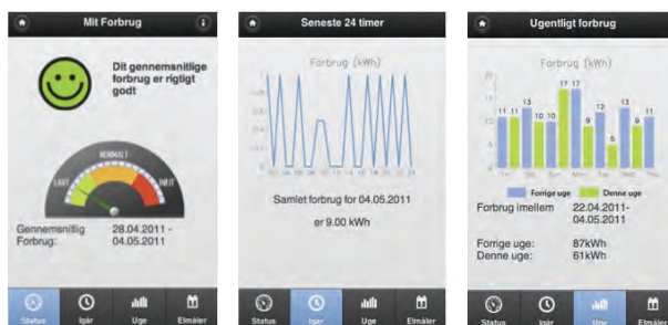
Figure 2. Three views on power consumption namely last week (injunctive), last week consumption (descriptive), and last week compared to the week before (descriptive).
