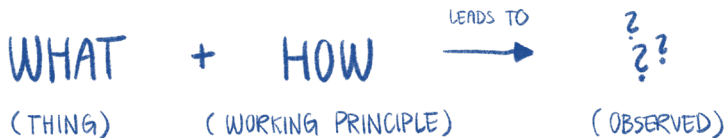
Figure 4: Equation for deduction; the only unknown is the result which is found by two known variables to the right of the arrow. This type of equation is the simplest since solving the equation does not require any rearranging of variables to arrive at a result. Model adopted from Dorst (2011).
