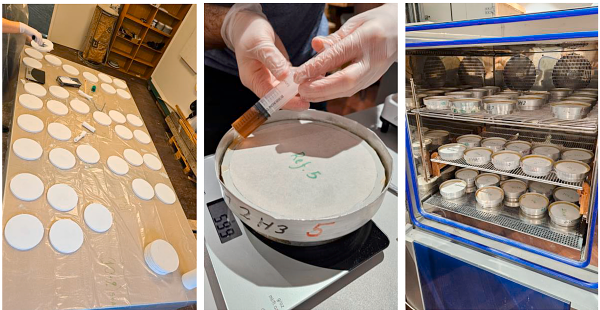
Fig. 4. Cup experiment: (a) Paint treatment of gypsum board disks, (b) Sealing test cups with mixture of beeswax and paraffin, (c) Placement of test cups inside climate chamber.
