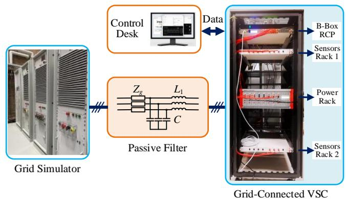
Fig. 22. A down-scale three-phase LC-filtered converter.
