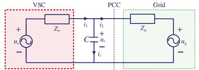
Fig. 2. Impedance model of grid-forming VSC.
