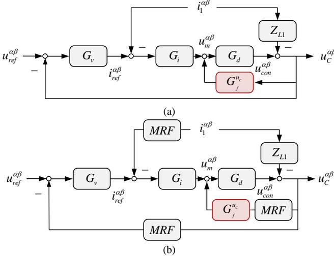
Fig. 14. Block diagram for voltage control in three-phase grid-forming VSCs with capacitor voltage feedforward damping.
