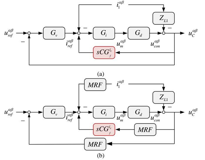
Fig. 11. Block diagram for voltage control in three-phase grid-forming VSCs with capacitor current feedforward damping.
