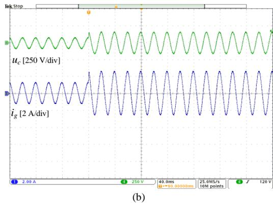
Fig. 28. Experimental results of a voltage transient ( $f_{LC}$  is lower than  $f_{cr}$  with double-sampling control). (a) Grid current feedforward damping with double-sampling. (b) Capacitor voltage feedforward damping with sixteen-sampling.
