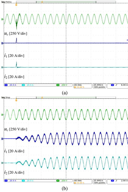
Fig. 24. Experimental results of dual-loop voltage control when  $f_{LC}$  is higher than  $f_{cr}$  with double-sampling control. (a) Grid current feedforward damping with double-sampling. (b) Capacitor voltage feedforward damping with sixteen-sampling.
