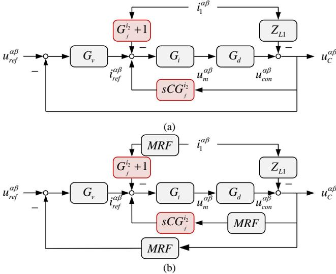
Fig. 7. Block diagram for voltage control in three-phase grid-forming VSCs with grid current feedforward damping. (a) With regular sampling control. (b) With multi-sampling control.
