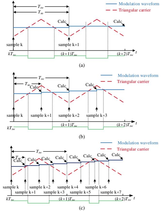
Fig. 4. Digital PWM with different sampling rates. (a) Single-sampling PWM. (b) Double-sampling PWM. (c) Multi-sampling PWM.
