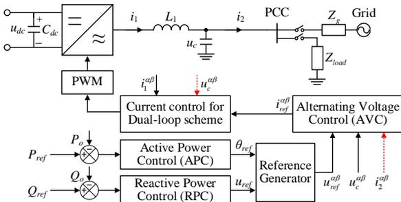
Fig. 1. The system overview of a three-phase grid-forming VSC.
