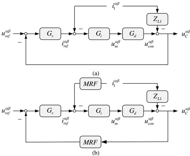
Fig. 3. Block diagram for voltage control for in three-phase grid-forming VSCs without feedforward damping. (a) With regular sampling control. (b) With multi-sampling control.
