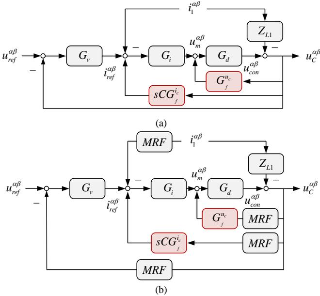
Fig. 17. Block diagram for voltage control in three-phase grid-forming VSCs with capacitor voltage feedforward damping and capacitor current feedforward damping.
