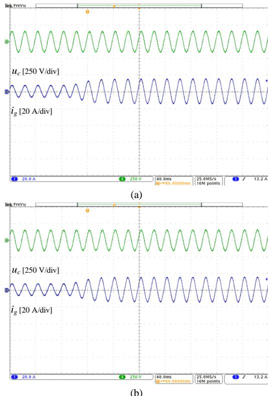
Fig. 27. Experimental results of a power transient ( $f_{LC}$  is lower than  $f_{cr}$  with double-sampling control). (a) Grid current feedforward damping with double-sampling. (b) Capacitor voltage feedforward damping with sixteen-sampling.
