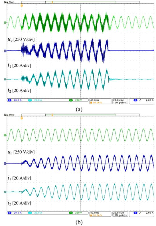
Fig. 26. Experimental results of voltage control considering a -20% parameter deviation of  $LC$ -filter and  $f_{LC}$  is lower than  $f_{cr}$  with double-sampling control. (a) Grid current feedforward damping with double-sampling. (b) Capacitor voltage feedforward damping with sixteen-sampling.
