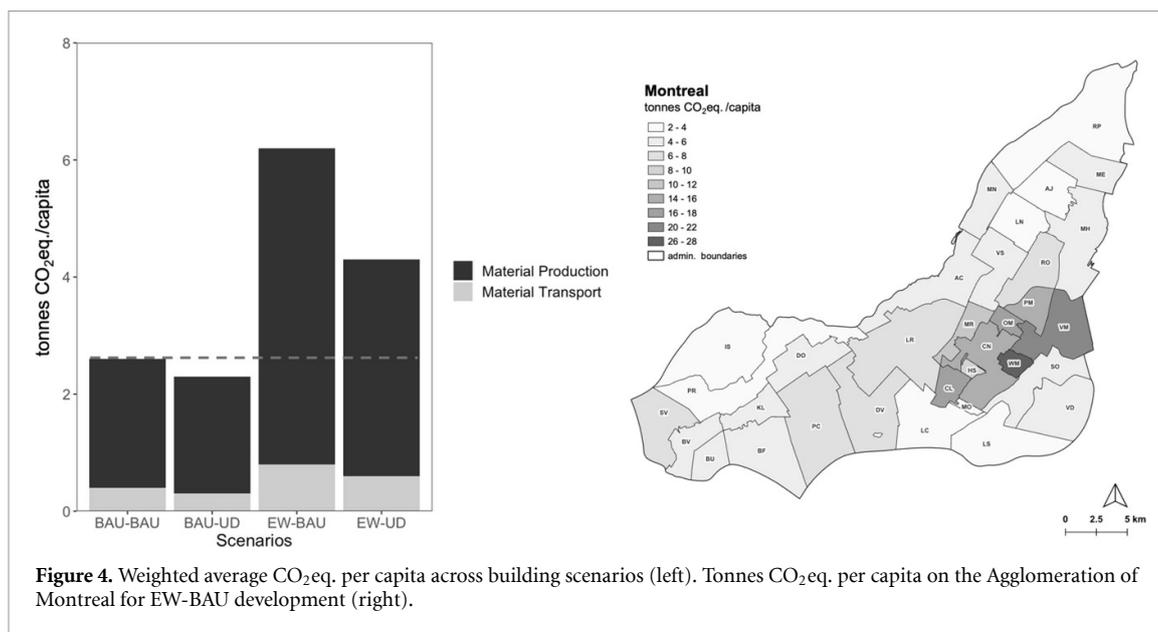
**Figure 4.** Weighted average CO<sub>2</sub>eq. per capita across building scenarios (left). Tonnes CO<sub>2</sub>eq. per capita on the Agglomeration of Montreal for EW-BAU development (right).
