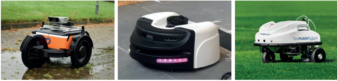
Figure 3.3: From Paper 1: Capra Robotics' Hircus, Coalescent Mobile Robotics' Serena (lab demo), and TinyMobileRobots' TinyLineMarker Sport. Disclosure is accepted.
