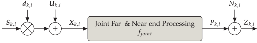
Fig. 11: Signal Model with joint far- and near-end speech and listening enhancement.
