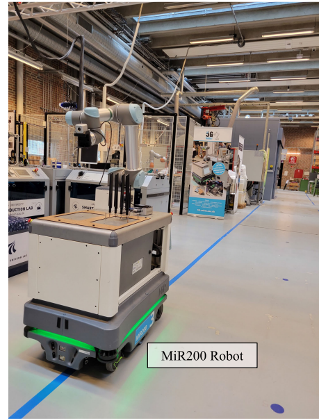
FIGURE 6. MiR200 AMR within the 5G Smart Production Lab.
