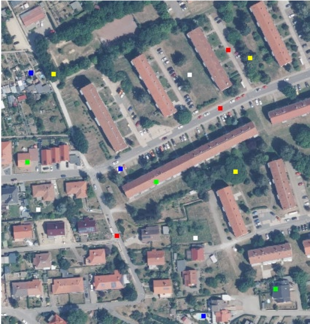
Fig. 1 Ortho-image and patches of pixels for the selected classes (green: 'building', red: 'impervious surface': white: 'low vegetation', yellow: 'tree', blue: 'clutter/background') for the derivation of the DT.
