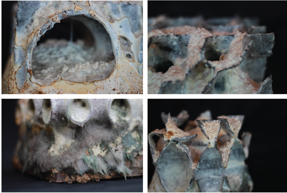
Figure 9: Details of resulting bricks after being impregnated with mycelium, and baked.
