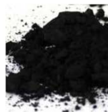
Black iron oxide Pigment The recipe is for the pigment to be made into a paste with water, and then added to the plaster. Soaking the pigment over-night may make the colour stronger.
