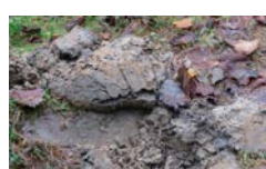
Moraine clay As a binder for clay plasters and floors
