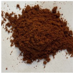
Sample of sand taken from the same location as above, but within the small dug hole, there was this redder deposit of sand. This material contains more iron-oxide than the sample above, but is otherwise identical.
