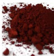
Red iron oxide Pigment The recipe is for the pigment to be made into a paste with water, and then added to the plaster. Soaking the pigment over-night may make the colour stronger.
