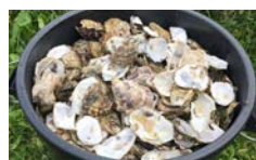
Shell material For floor sub-base
