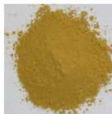
Yellow iron oxide Pigment The recipe is for the pigment to be made into a paste with water, and then added to the plaster. Soaking the pigment over-night may make the colour stronger.
