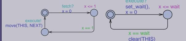
**Fig. 7:** Pipeline fetch and execute stage, respectively.
